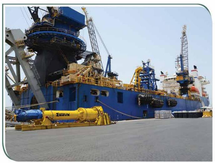
This vessel is a Rigid pipe S-lay and Heavy lift DP-2 construction vessel with the main features of DP-3. Designed for work in both deep and shallow water, the Global 1201 has an A&R winch capacity of 400 MT
